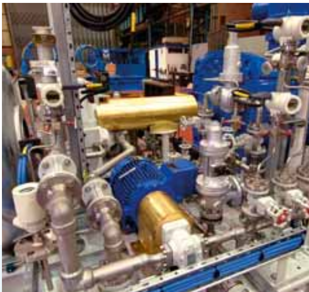
Protection Devices: Optional API lubrication system
