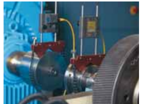
Coupling alignment: Laser alignment of gearbox and motor shafts
