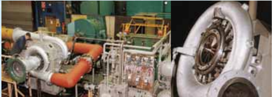
Testing: Performance testing of blowers to international codes at our Renfrew works
