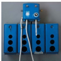
830GAP-Q1G 1 gpm four chemical Dial-A-Blend (4 liters/minute) 4 gpm single product bucket fill (16 liters/minute) Four 1 gallon/5 liter locking enclosures
