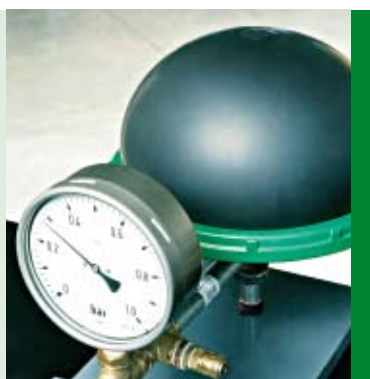
Testing the physical strength of imperforated membranes
