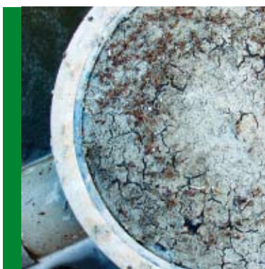
Clogged membrane before cleaning (courtesy of Dr.-Ing. Frey)
